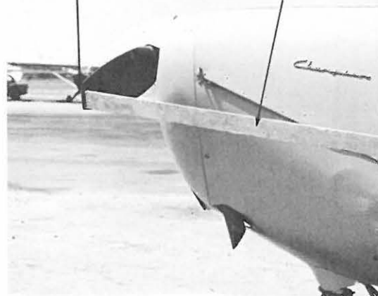
FIG. 21-12 Checking the track of a metal propeller on an airplane.
