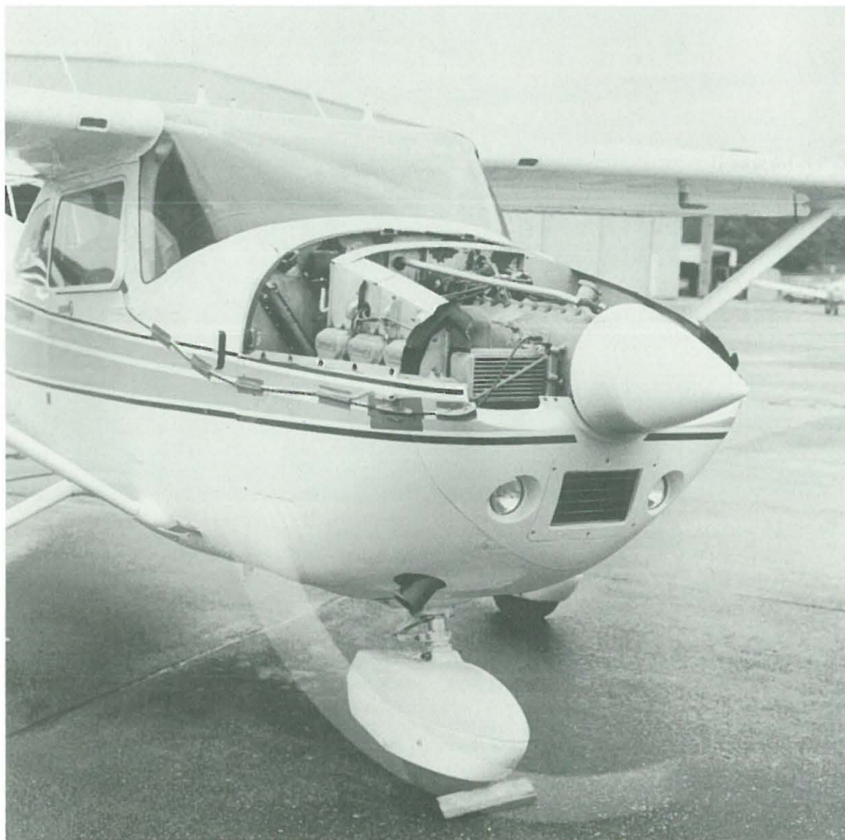
FIG. 21-20 Cable and transducer installation for balancing. (Dynamic Solutions Systems, Inc.)
