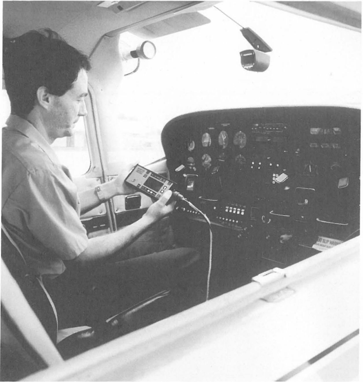
FIG. 21-21 Collection of balancing data during ground run-up. (Dynamic Solutions Systems, Inc.)
