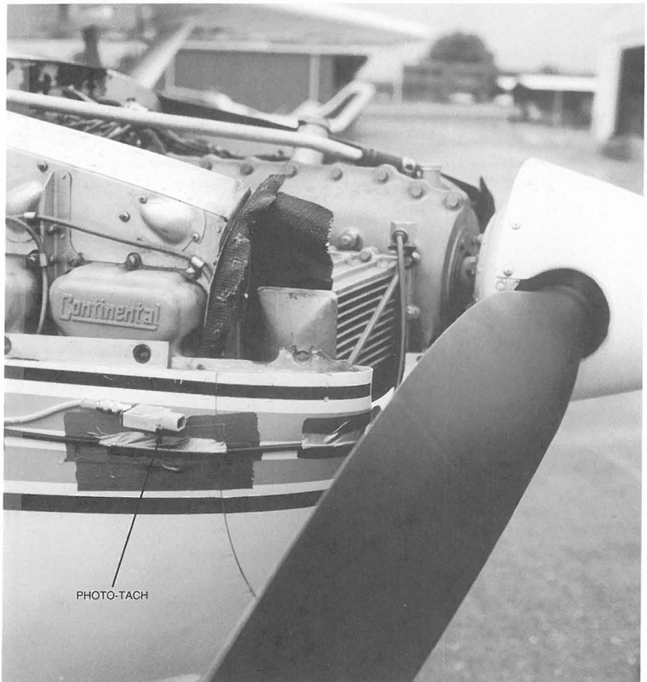
FIG. 21-19 Photo-tach installation for balancing. (Dynamic Solutions Systems, Inc.)
