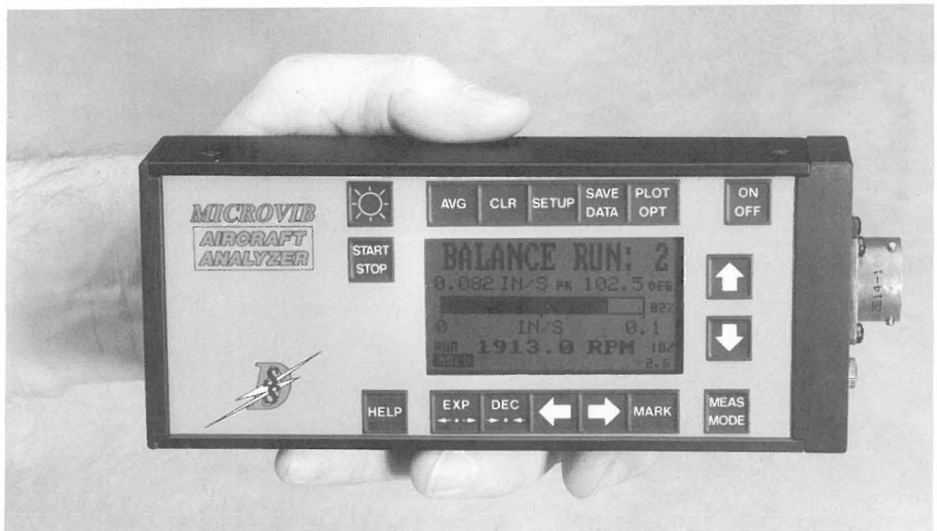
FIG. 21-17 Micro-Vib aircraft vibration analyzer/balancer. (Dynamic Solutions Systems, Inc.)
