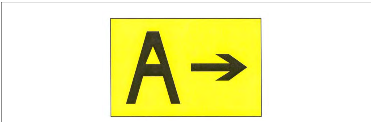
FIG 2-3-36 Direction Sign for Runway Exit
