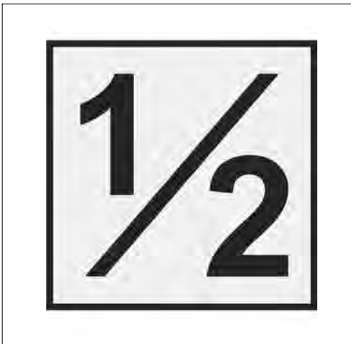
FIG 7-5-1 Typical Runway Half-way Sign
